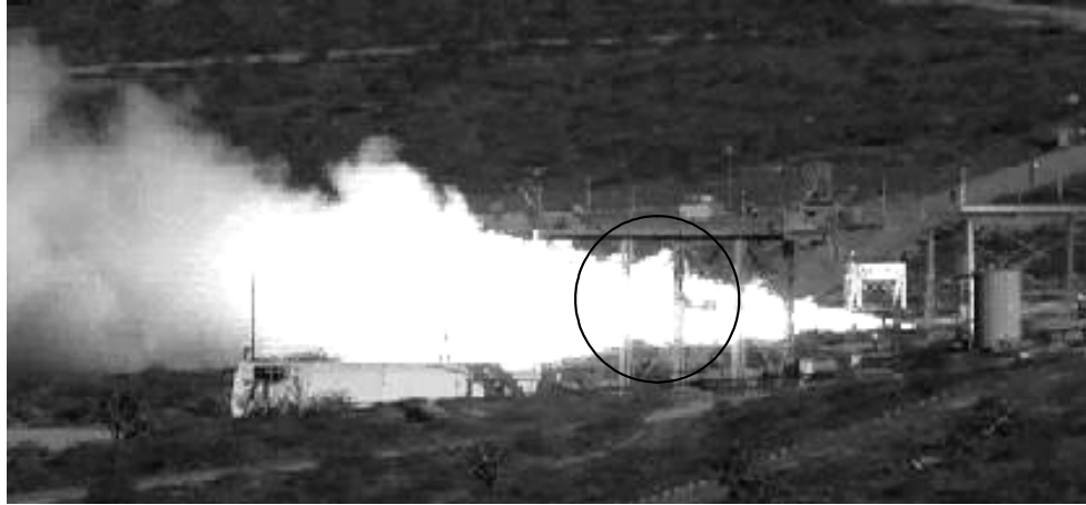
Figure 3.8: Photo of SRM test. The motor is laying horizontally with the nose pointed to the right in this view. The actual body of the motor is hidden from view by a protective berm. The black circle indicates the approximate FOV of the spectrometer.
