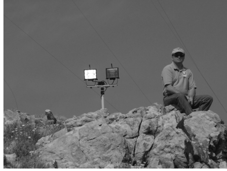
Figure 3.6: Photo of experimental setup for QTH observations at Edwards AFB, taken from the spectrometer location. Photo shows the QTH lamp and AFIT technician Greg Smith (right). Greg is not within the instrument FOV in this photo.
